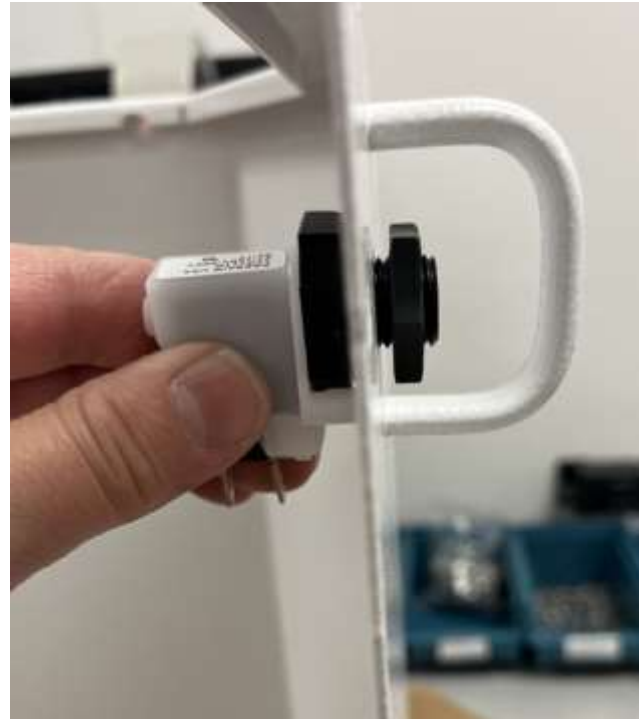
Picture of air switch assembled onto front of aspirator bottom cover
