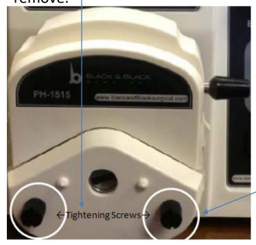
To install new pump head, line up pump head notch with grommet on motor inside of pump and carefully push in. Secure head by tightening the 2 tightening screws.
