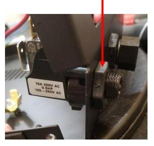
Remove damaged switch
