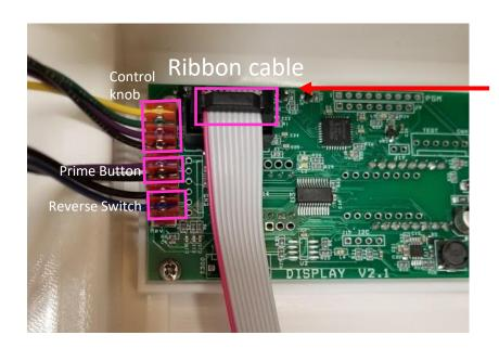
Remove 4 sets of cables from display board
