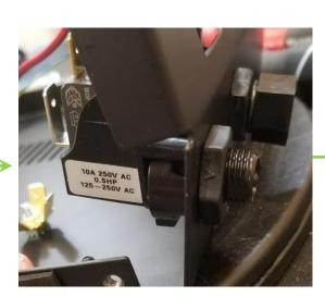
Secure tightening nut
